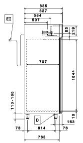
FΙ Electrical inlet (power) Refriaerant Inlet Refrigerant Outlet
